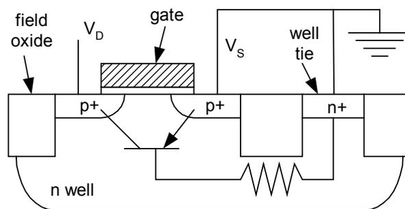
Figure 3: Cross section schematic of p channel MOS transistor showing parasitic pnp bipolar transistor and n well resistor connection to the base of the parasitic bipolar.
