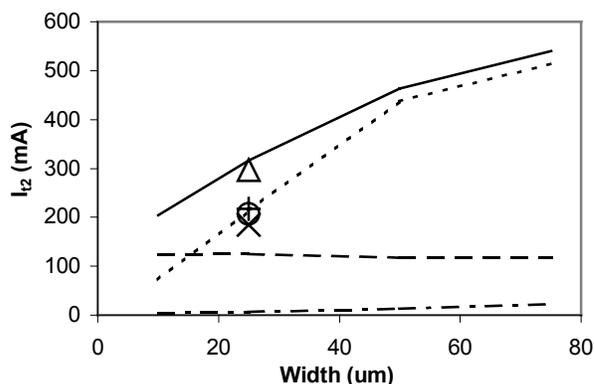
Figure 10: . Five site averages of  $I_{t2}$  for snapback devices of various geometries. Table 1 explains symbols.
