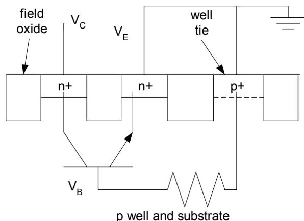
Figure 11: Cross section schematic of a snapback device showing the parasitic npn bipolar.
