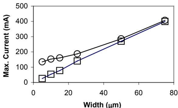
Figure 15: Current carrying capability of GDNTR in series with an n channel transistor as a function of width. Points are the average of 4 sets of data on a wafer. □  $I_{l2}$  defined by kink in I-V curve, ○  $I_{l2}$  defined by 0.1  $\mu$ A of leakage.
