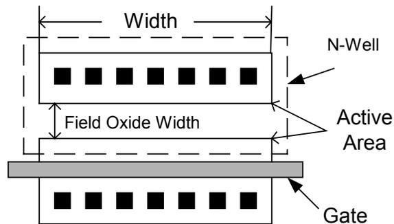
Figure 12: Layout of a field oxide defined n well resistor integrated with an n channel transistor.
