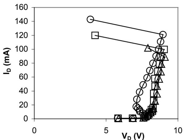
Figure 2: TLP I-V curve of 3.3V pchannel transistors.  $\circ$  10  $\mu\text{m}$  well tie,  $\square$  0.24  $\mu\text{m}$  well tie with separate pads,  $\triangle$  0.24  $\mu\text{m}$  well tie shorted to the source in metal. All devices are 25  $\mu\text{m}$  wide with a drawn gate length of 0.28  $\mu\text{m}$ . The devices have minimum design rule separation between contacts and the gate. All voltages are negative.
