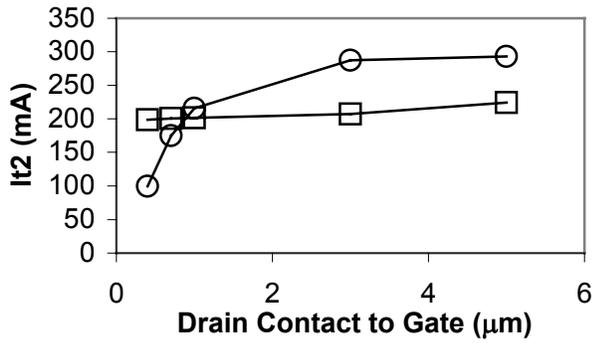
Figure 5:  $I_{t2}$  as a function of drain side contact to gate separation for 3.3 V,  $\circ$ , and 1.5 V,  $\square$ , n channel transistors. Results are average of 5 sites on a wafer. All transistors are 25  $\mu\text{m}$  wide and have drawn gate lengths of 0.16 and 0.32  $\mu\text{m}$  for the 1.5 V and 3.3 V transistors respectively.
