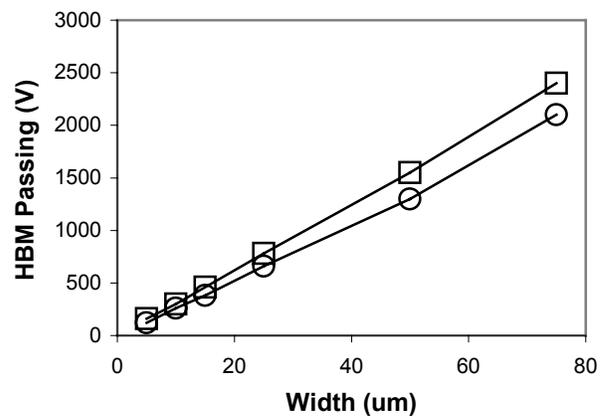
Figure 8: HBM measurements of n channel transistors.  $\square$  1.5 V transistors,  $\circ$  3.3 V transistors
