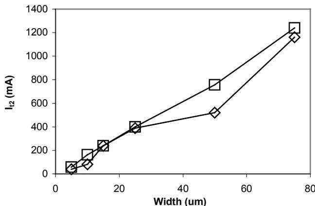
Figure 9:  $I_{t2}$  as a function of width for 1.5 V n channel transistors with gate shorted to the source.
