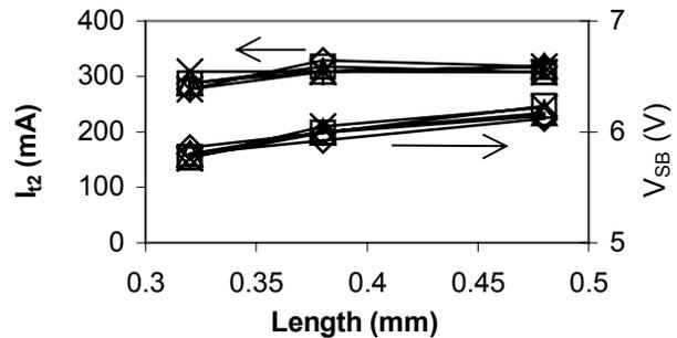
Figure 6:  $I_{t2}$  as a function of transistor length for 3.3V n channel transistors.
