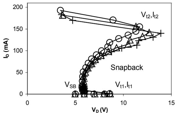
Figure 14: Sample TLP measurements for GDNTR integrated with an n channel transistor. The device is 25  $\mu\text{m}$  wide with GDNTR gate lengths of  $\circ$  0.20  $\mu\text{m}$ ,  $\Delta$  0.28  $\mu\text{m}$ , and  $+$ , 0.36  $\mu\text{m}$ .
