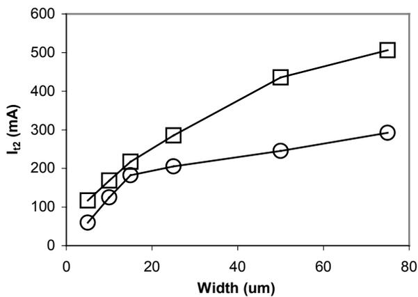
Figure 7:  $I_{t2}$  as a function of width for n channel transistors.  $\square$  3.3 V,  $\circ$  1.5 V
