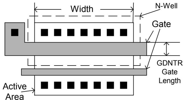
Figure 13: Layout of a gate defined n well resistor integrated with an n channel transistor. The contact to the gate is tied in metal to the contacts to the active area inside the n well.
