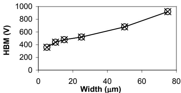
Figure 16: HBM data for two sets of packaged test structures of GDNTR in series with n channel transistors.
