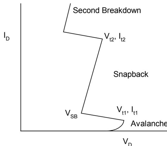
Figure 1: Schematic I-V curve of snapback.
