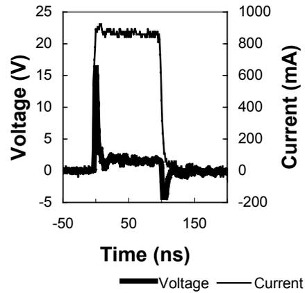
Figure 6. Voltage and current waveform into a short circuit.
