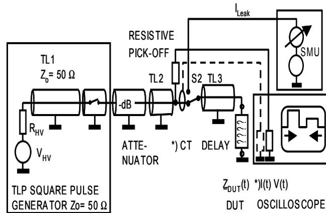
Figure 2: Time Domain Reflectometer (TDR) TLP with attenuator for re-reflected stress pulses.
