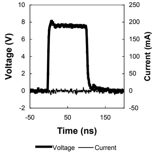
Figure 5. Voltage and current waveform into an open-circuit.
