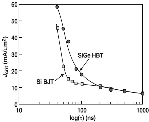
Figure 10. Critical current-to-failure of a Si BJT and SiGe HBT device
