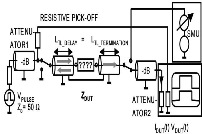
Figure 4: Time Domain Reflection & Transmission TLP (TDRT) without attenuation of the re-reflected stress pulse
