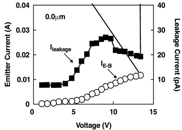
Figure 9. TLP I-V and leakage characteristic of a transistor.
