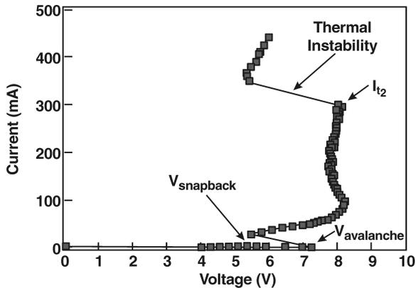
Figure 8. TLP I-V characteristic highlighting the key transition points.
