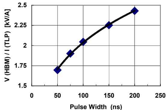
Figure 12. HBM-TLP Correlation as a function of pulse width.
