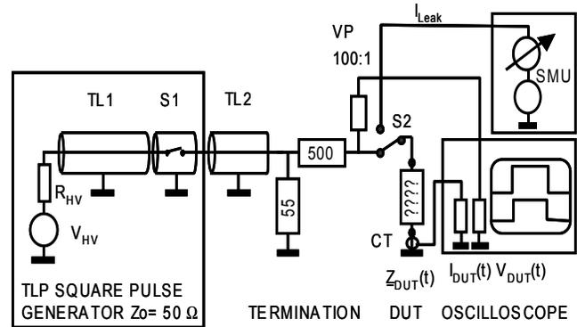
Figure 1: TLP Current Source Configuration.
