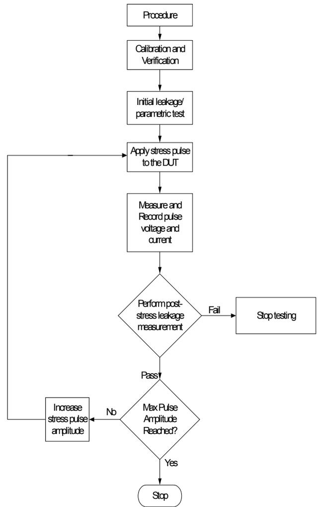
Figure 7. TLP Testing Sequence and Method.
