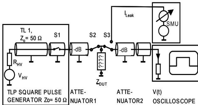
Figure 3: Time Domain Transmission (TDT) TLP system without attenuation of stress pulses reflected from the open end of the TL1.
