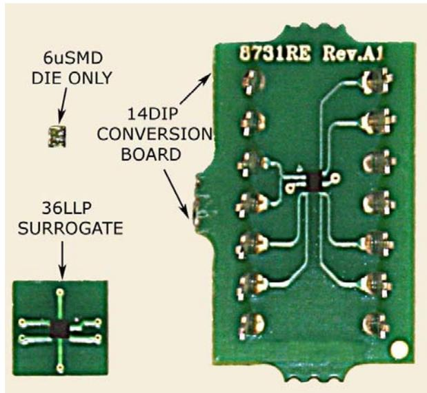
Figure 13. From left to right: 6 $\mu$ SMD (top left) package only; 36LLP surrogate (bottom left) with 6 $\mu$ SMD mounted on it; 14DIP conversion board (right) with 6 $\mu$ SMD mounted on it.
