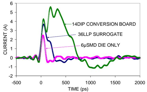
Figure 14. Waveform comparison for chip-scale package (6 $\mu$ SMD) vs 36 LLP (QFN) Surrogate vs 14 DIP Conversion Board at 500V with 8 GHz oscilloscope.
