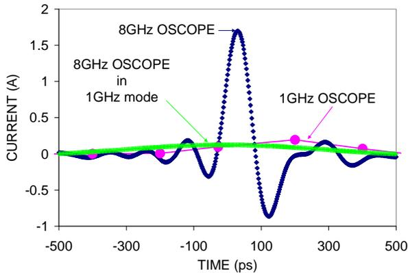
Figure 2. Comparison of FCDM waveforms for 6µSMD (CSP) package with 8 GHz oscilloscope, 8 GHz oscilloscope in 1 GHz mode and 1 GHz oscilloscope at 500 V CDM stress.
