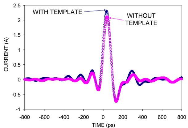
Figure 12. Waveform comparison with and without support template (6LLP at 500 V with 8 GHz oscilloscope)
