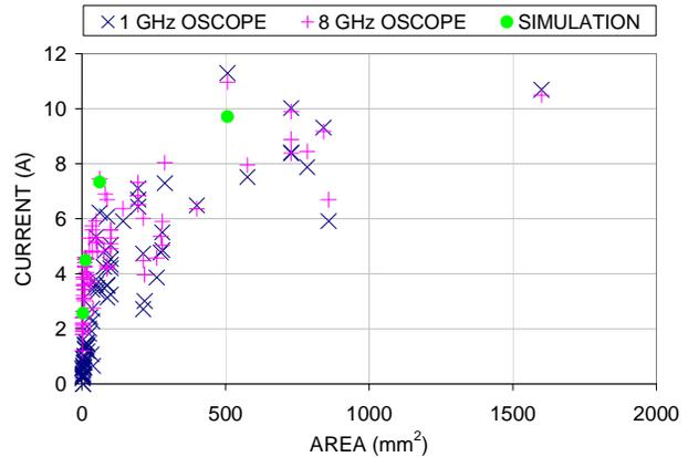
Figure 3. Peak current versus area for all packages tested for this study
