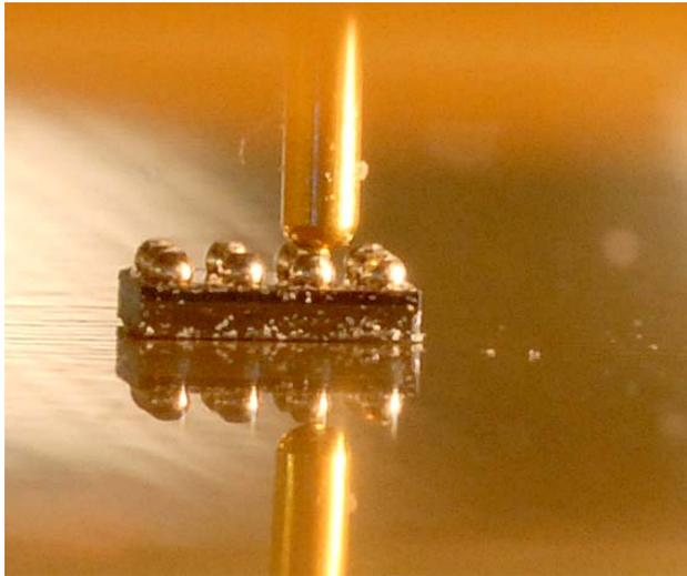
Figure 10. Unconstrained Chip Scale Device in CDM tester (ORION)
