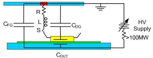
Figure 7. Three capacitor FCDM model
