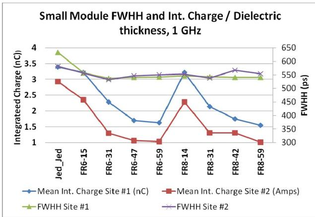
Figure 12. Small module FWHH and integrated charge as a function of dielectric thickness, 1 GHz measurement.
