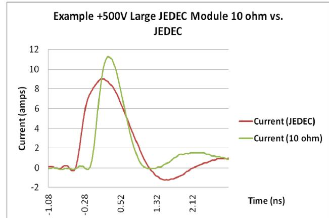
Figure 4. Example +500V 3 GHz JEDEC large module waveforms comparing 10 ohm CDM to JEDEC CDM.
