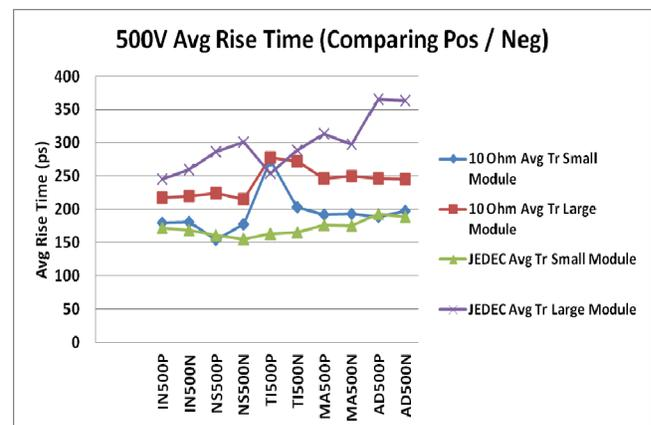
Figure 5. Average 10 ohm vs. JEDEC 3 GHz oscilloscope bandwidth rise time between sites measured at 500V.
