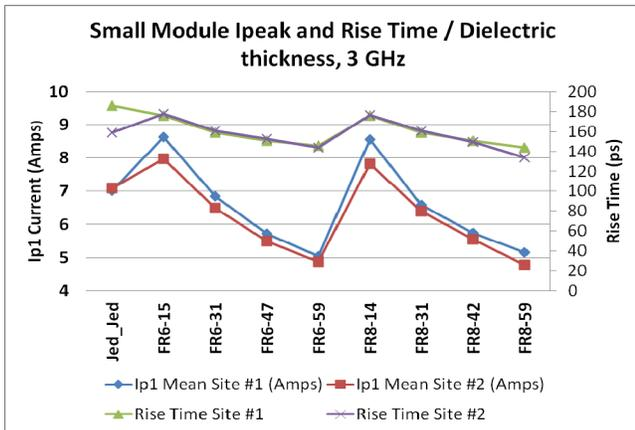
Figure 13. Small module Ipeak and risetime as a function of dielectric thickness, 3 GHz measurement.
