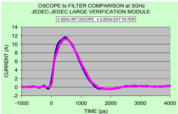
Figure 10. DPO70804 oscilloscope waveform comparison of 3 GHz internal software filter (dark) and external hardware filter (right).
