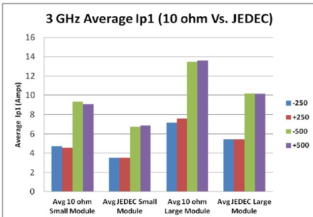
Figure 3. Average first peak current at 3 GHz comparing 10 ohm CDM to JEDEC CDM.
