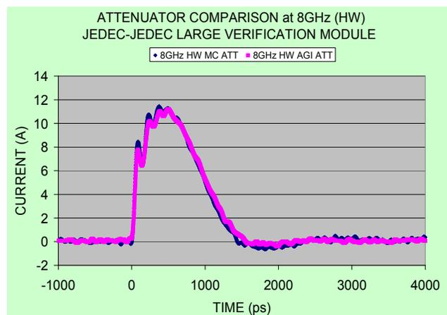
Figure 8. DPO70804 oscilloscope 8 GHz waveforms comparing different 18 GHz 20 dB attenuators.
