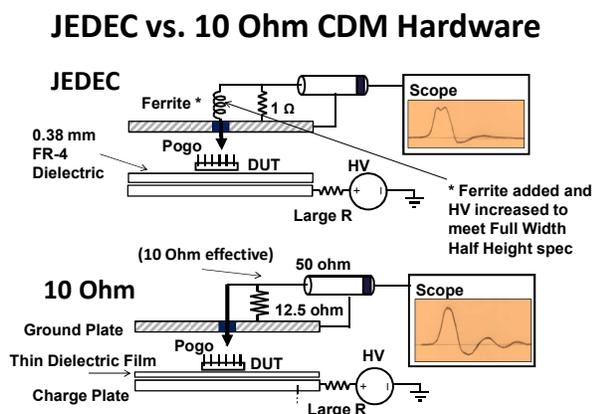
Figure 1. JEDEC CDM and 10 ohm CDM hardware schematics.
