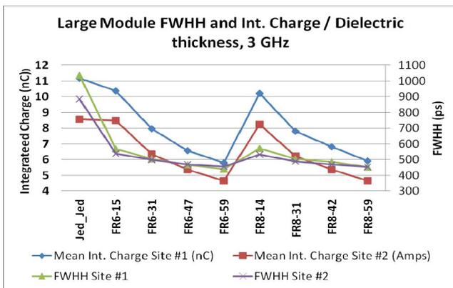
Figure 18. Large module FWHH and integrated charge as a function of dielectric thickness, 3 GHz measurement.
