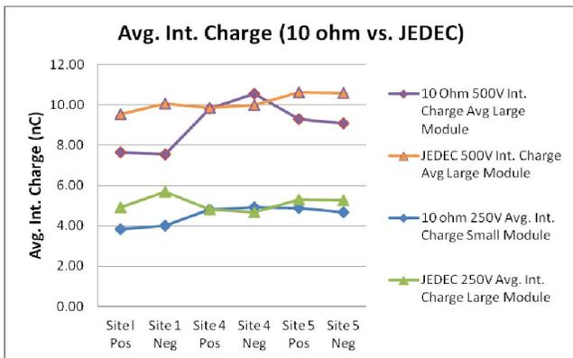
Figure 7. Average 10 Ohm vs. JEDEC 3 GHz integrated charge between sites comparing at 250V and 500V.
