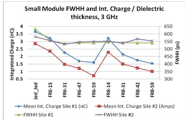
Figure 14. Small module FWHH and integrated charge as a function of dielectric thickness, 3 GHz measurement.
