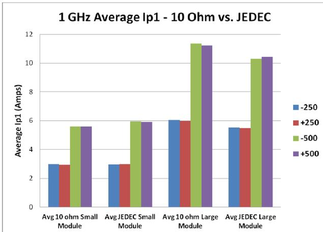
Figure 2. Average first peak current at 1 GHz comparing 10 ohm CDM to JEDEC CDM.
