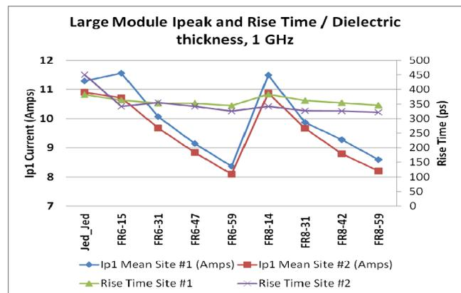
Figure 15. Large module Ipeak and rise time as a function of dielectric thickness, 1 GHz measurement.
