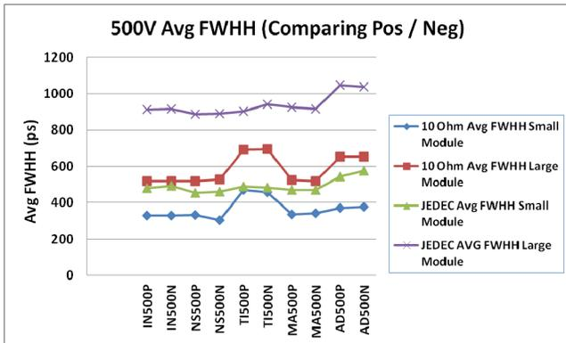
Figure 6. Average 10 ohm vs. JEDEC 3 GHz oscilloscope bandwidth full width at half height (FWHH) between sites measured at 500V.
