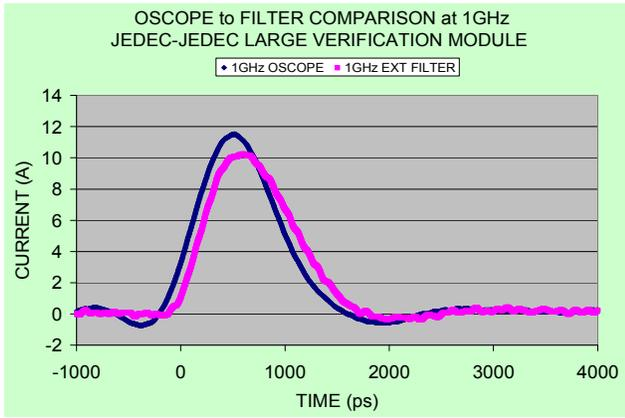
Figure 9. DPO70804 oscilloscope waveform comparison of 1 GHz internal software filter (dark) and external hardware filter (right).
