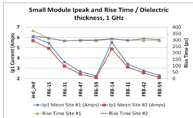
Figure 11. Small module Ipeak and rise time as a function of dielectric thickness, 1 GHz measurement.
