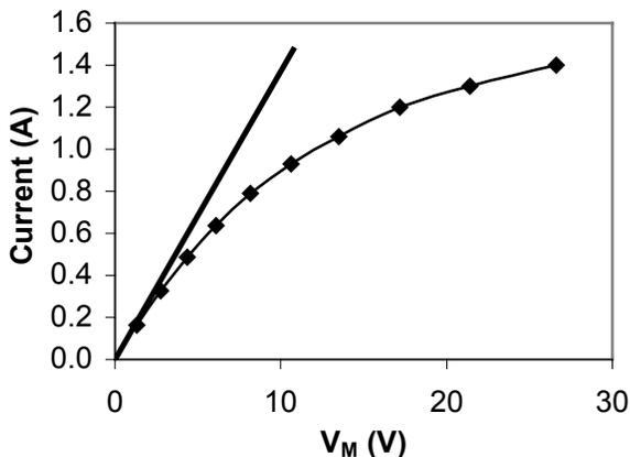
Figure 4 TLP and DC measured I-V curve of a 60 X 60 mm gate resistor.
