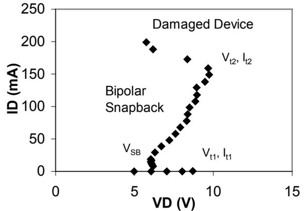
Figure 1 Sample TLP Data for an nMOS transistor. Shows junction breakdown,  $V_{t1}$ , bipolar snapback holding voltage  $V_{SB}$ , second breakdown point,  $V_{t2}$ , and region of device damage.
