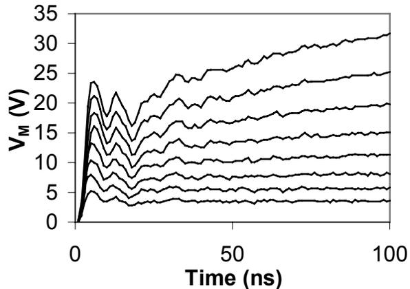
Figure 5 Voltage as a function of time for charging voltages of 20 to 90 V in 10 V steps for a 60 X 60  $\mu\text{m}$  gate structure using low impedance system
