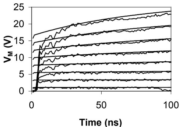
Figure 11 Voltage as a function of time for charging voltages of 5 to 75 V in 10 V steps for a 1.5 X 60  $\mu\text{m}$  gate structure using high impedance system.
