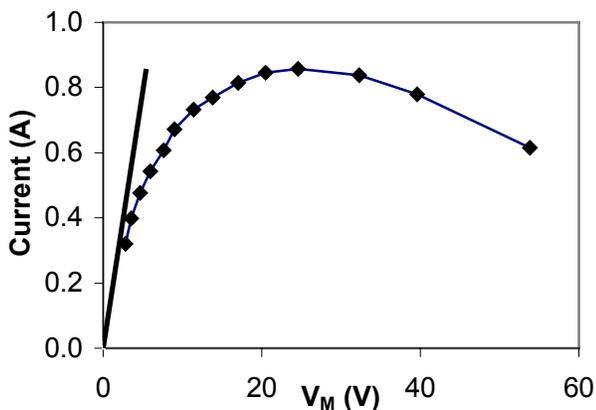
Figure 3 TLP and DC measured I-V curves of copper resistor 213  $\mu\text{m}$  long and 3  $\mu\text{m}$  wide.
