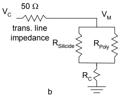
Figure 7 DC equivalent circuits of high and low impedance TLP systems with gate resistance and contact resistance.
