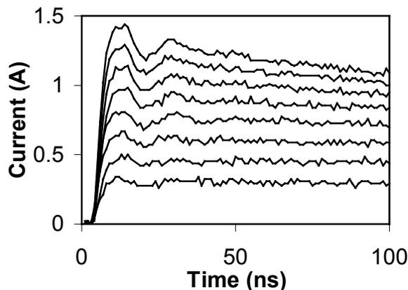
Figure 6 Current as a function of time for charging voltages of 20 to 90 V in 10 V steps for a 60 X 60  $\mu\text{m}$  gate structure using low impedance system.
