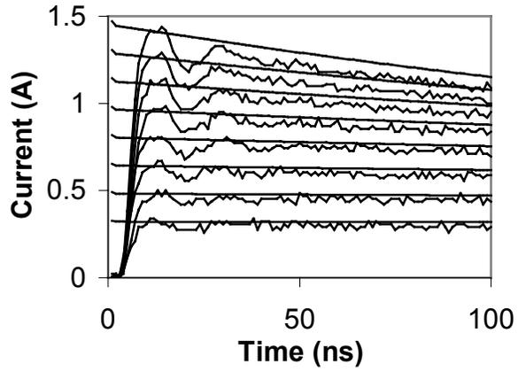
Figure 10 Current as a function of time with model calculations added. Same data as Figure 6.
