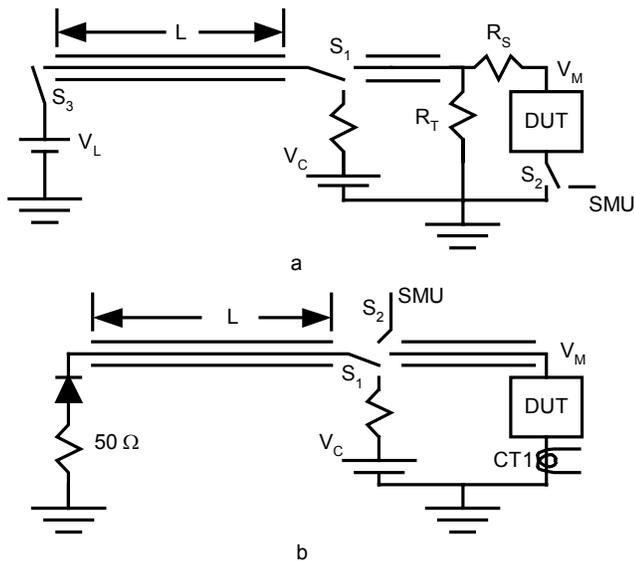
Figure 2 Schematics of high (a) and low (b) impedance TLP systems.
