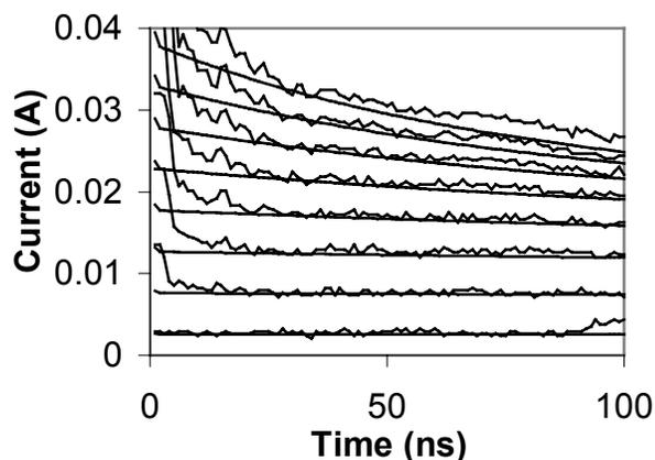
Figure 12 Current as a function of time for charging voltages of 5 to 75 V in 10 V steps for a 1.5 X 60  $\mu\text{m}$  gate structure using high impedance system.
