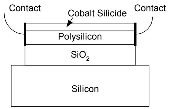
Figure 8 Geometry used for resistance model
