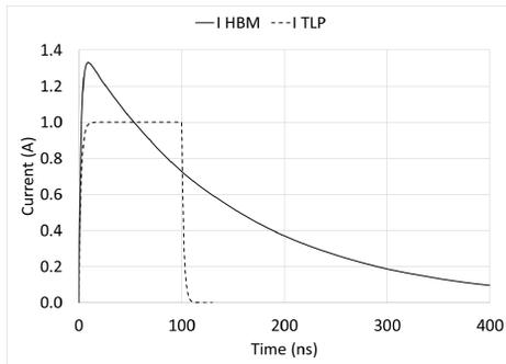
Fig. 3 Comparison of a 2000 V HBM pulse with a 1 A 100 ns long TLP pulse
