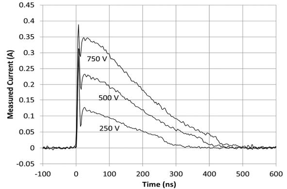
Fig. 6 Current versus time for the three HBM pulse on the nLDMOS
