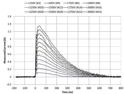
Fig. 10 Current versus time measurements on select HBM pulses for SCR Design 1
