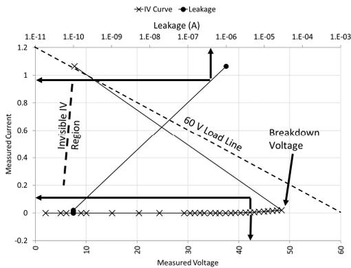
Fig. 5 TLP IV and leakage measurements on the nLDMOS transistor test structure as well as the load line for the final TLP pulse
