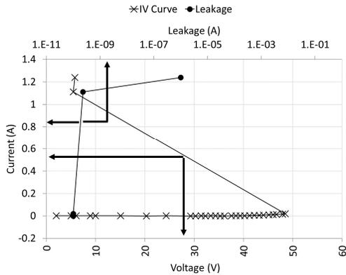
Fig. 13 TLP measurements of SCR Design 2
