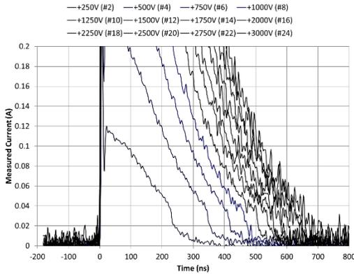
Fig. 12 HBM current versus time for SCR Design 1 with an expanded current scale
