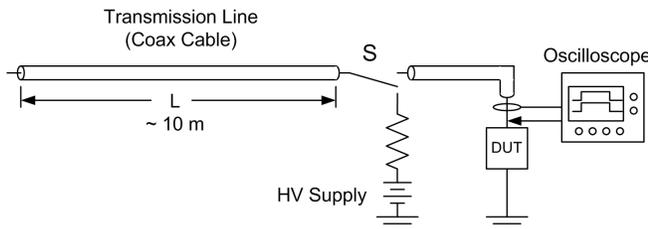
Fig. 2 Simplified TLP schematic (elements to remove unwanted reflections are not shown)
