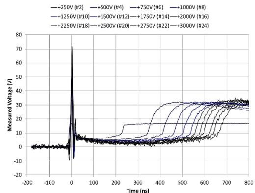
Fig. 11 Voltage versus time measurements on select HBM pulses of Field Oxide Device
