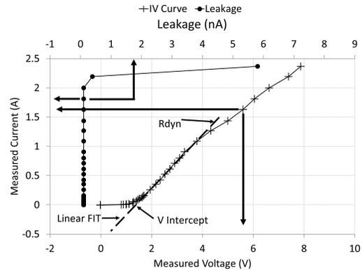
Fig. 4 TLP measurements of a p-NWell diode in forward bias. + marks are TLP IV points. ● marks are leakage measurements made after each TLP pulse. The arrows in this figure, and in the remaining TLP IV measurements, indicate the axes used for plotting each set of points. The y value for the leakage is the TLP pulse current for the pulse preceding the leakage measurement.
