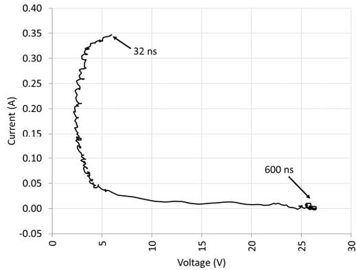
Fig. 8 IV curve of the nLDMOS device derived by plotting current versus voltage time point by time point starting at 32. ns into the pulse and ending at 600 ns
