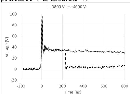
Fig. 16 Voltage capture on the 3800 V and 4000 V HBM pulses on the full protection design using the pnp structure
