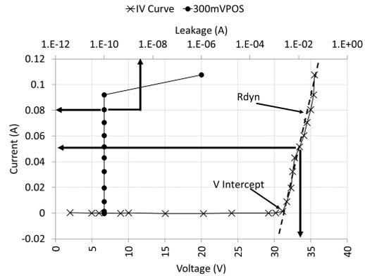
Fig. 14 TLP measurement of pnp device. The dashed line is a linear fit to the data over the range of 10 to 100 mA
