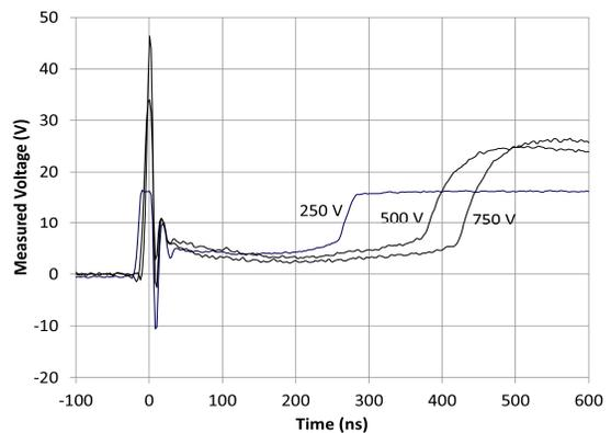
Fig. 7 Voltage versus time for the three HBM pulses on the nLDMOS
