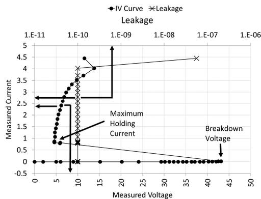
Fig. 9 TLP measurements of SCR Design 1. The device shows deep snapback and a failure at 4 A.
