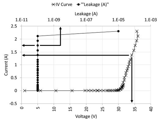
Fig. 15 TLP on full ESD protection structure using pnp devices
