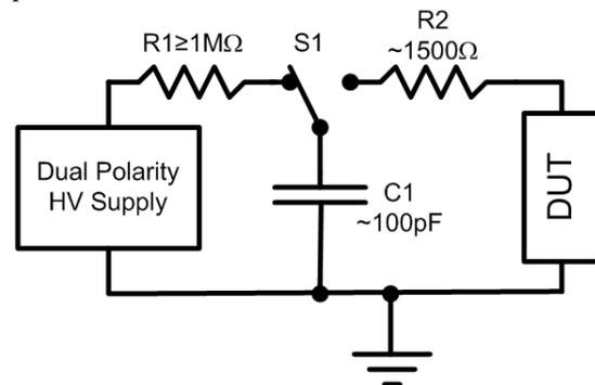
Fig. 1 Schematic of the HBM test
