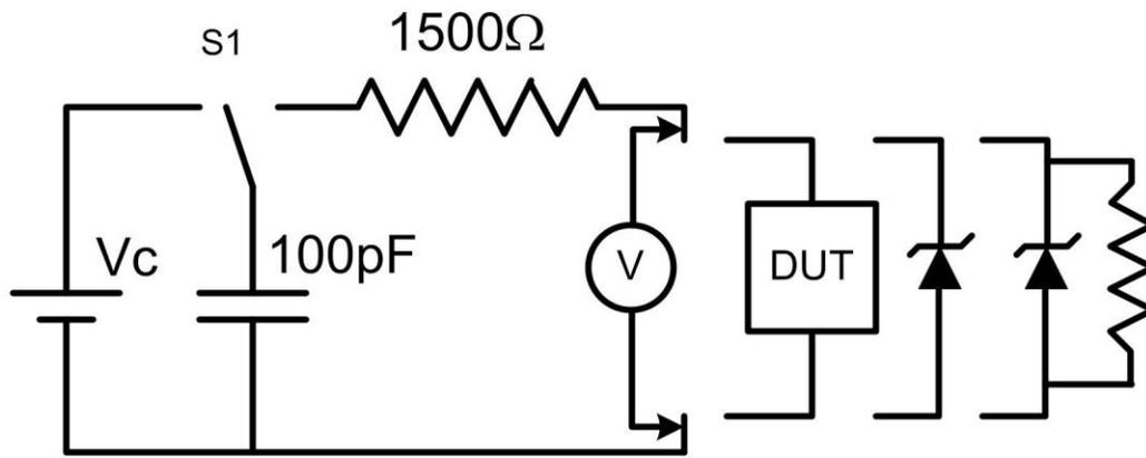
**Figure 1: Basic HBM schematic showing the location of the device under test, the positioning of the Zener diode and Zener diode with parallel resistors as well as the location of the voltage probe during measurement of the PPV**
