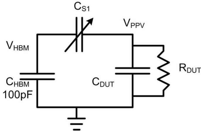
**Figure 4: Schematic for model of PPV due to relay capacitance change**
