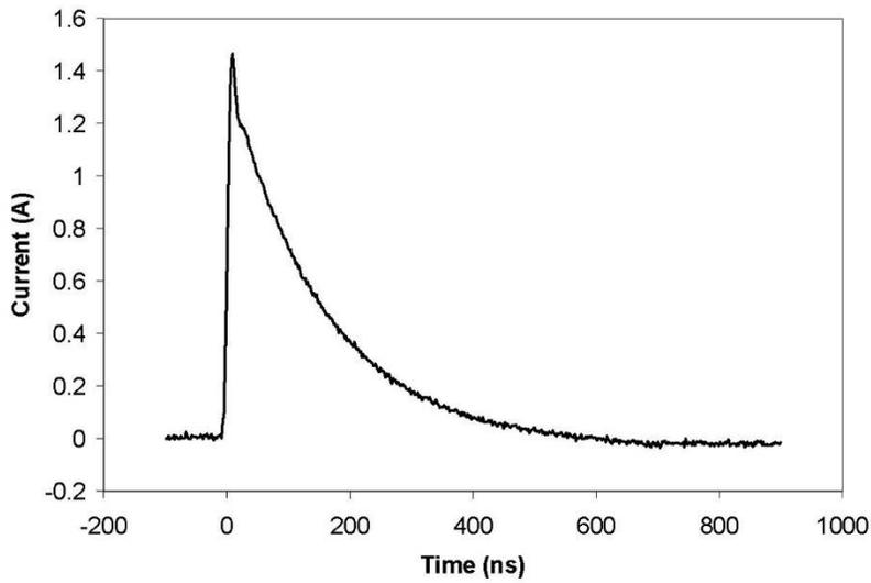
Figure 2: Measured HBM waveform for 2000V into a short
