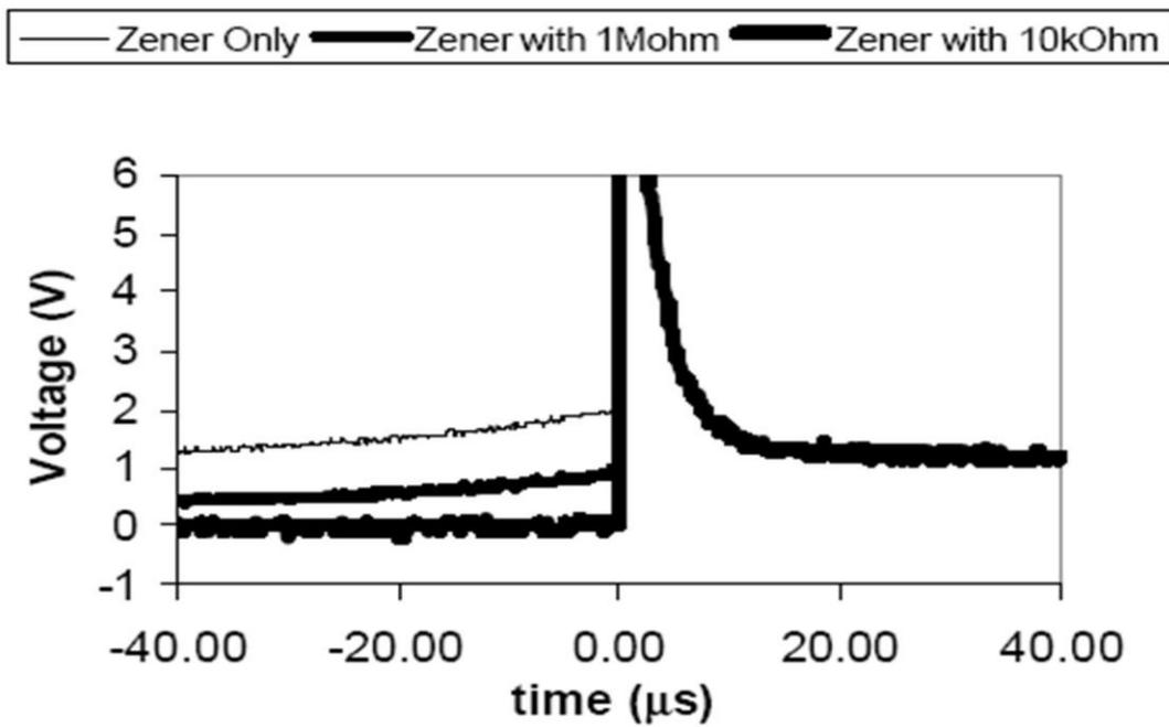
Figure 3: PPV measured across a 10V Zener diode and with  $1M\Omega$  and  $10k\Omega$  across the Zener
