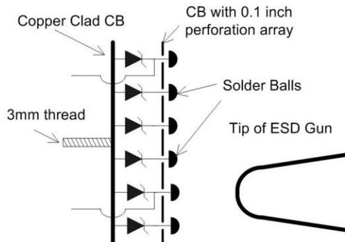
**Figure 6: Schematic of simulated integrated circuit**
