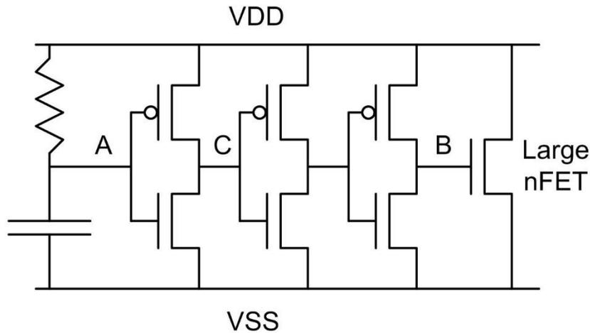
**Figure 5: Schematic of a typical dynamic ESD clamp**
