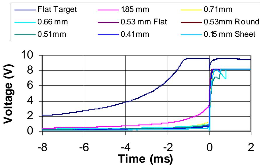
**Figure 8: Measured PPV for different geometry pins**
