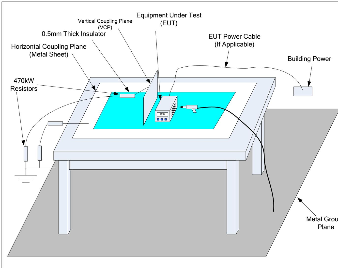
Figure 1 Test setup for ESD testing of small or table top systems as specified by IEC 61000-4-2.
