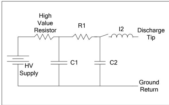
Figure 2 Schematic of an ESD gun
